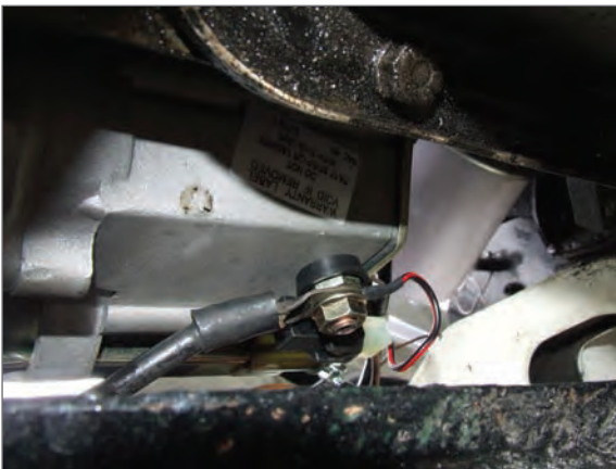
Picture 3: The main terminal viewed from underneath between sump and chassis.
