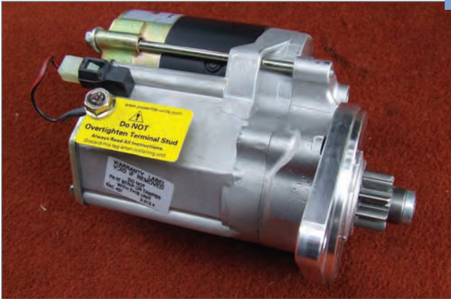
Picture 1: General view of unit showing the two electrical terminals and the connecting wire (left) and starter gear (right).
