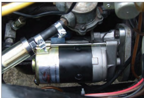
Picture 2: The motor installed. The supply cable can be seen running from centre right to centre bottom.
